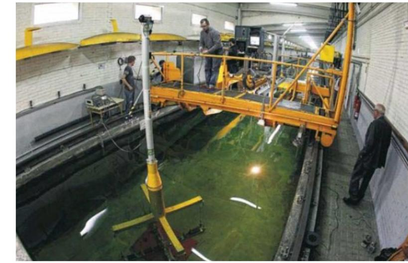
Channel test-bed for underwater inspection robots
